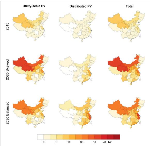
Figure 1. PV installed capacity (GW) by province for (a) 2015; (b) 2030 Skewed deployment (1:6 ratio of utility to distributed PV); and (c) 2030 Balanced deployment (1:1 ratio of utility to distributed PV).
